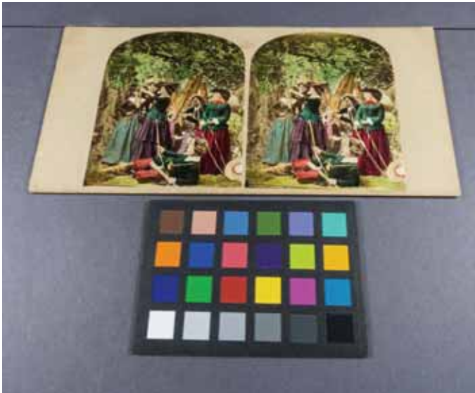
Image placement along a jig aligned to the camera field for primary photographic capture. Neutral photographic gray background and color standards facilitate high fidelity object documentation.
